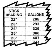
The easiest way to explain this procedure is with an example. Let's say you have a stick reading of 23d inches and you need to figure how many gallons are in your tank.
