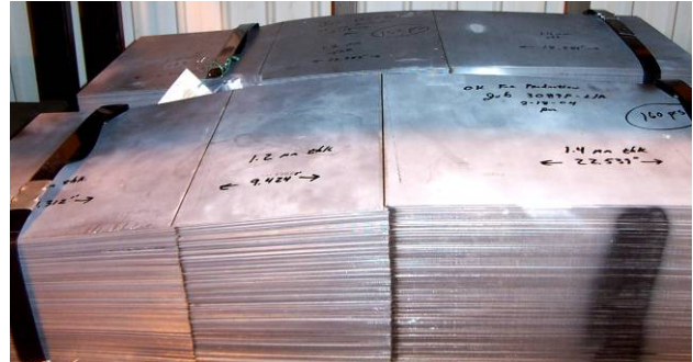
Figure 2. Rail inner and rail outer laser-welded blanks
