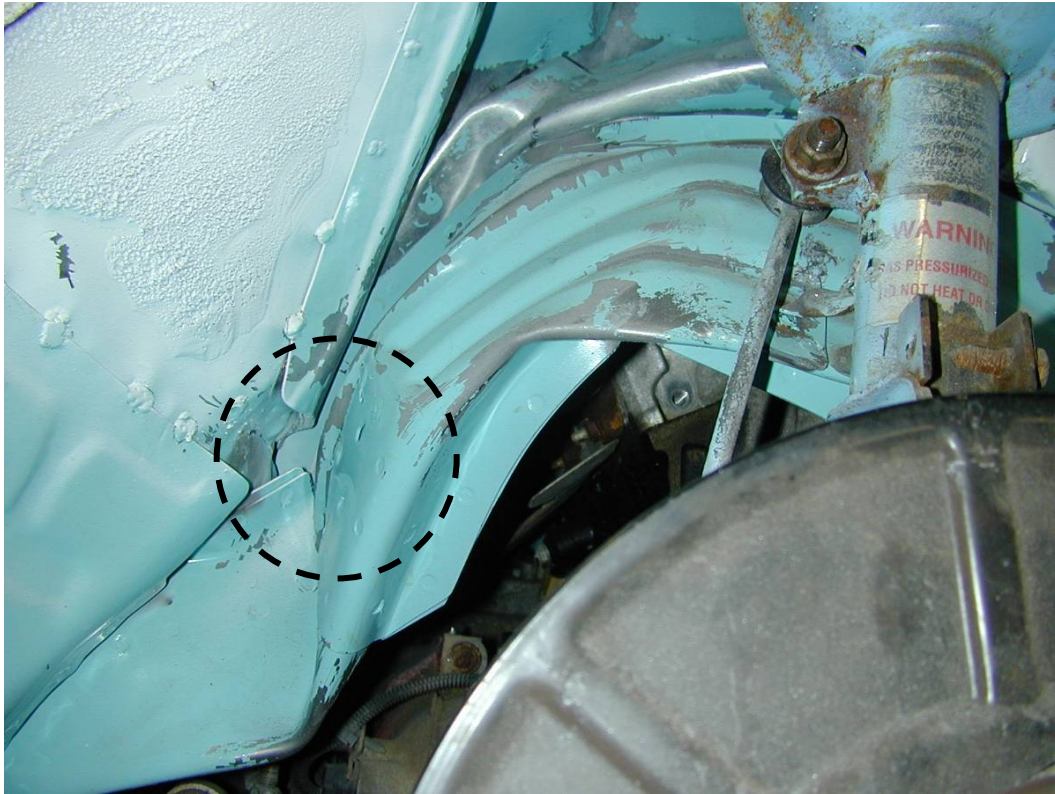
Photo 13. Slip joint with resistance spot and MIG puddle welds highlighted.
