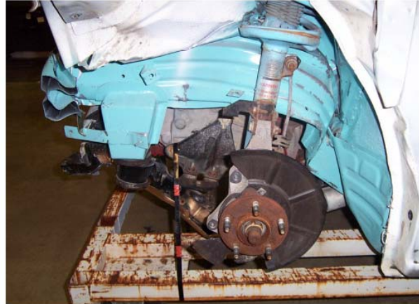
Photo 7. NCAP Test - Front Rail Views
