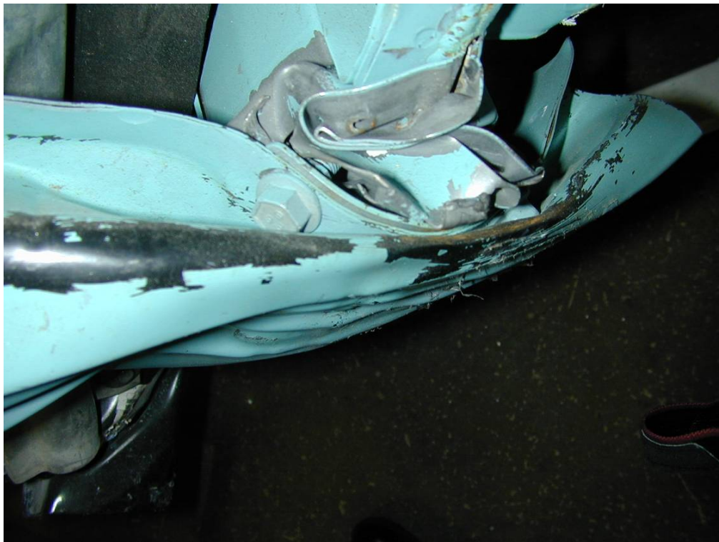
Photo 14. Left-hand rail-to-bumper reinforcement collapse. Weld buttons were pulled from the AHSS materials when separation was observed.
