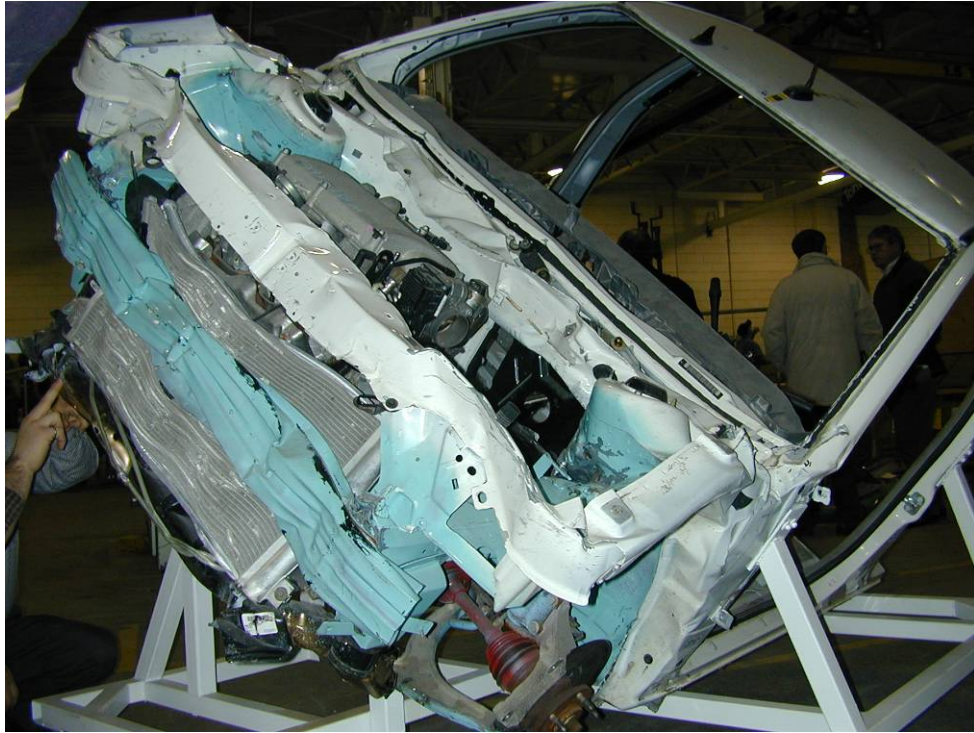
Photo 15. Front view showing bumper reinforcement and rail collapse. All welds were acceptable.
