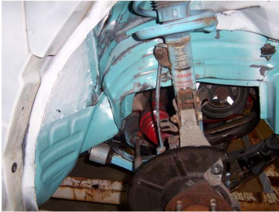
Photo 7. NCAP Test - Front Rail Views
