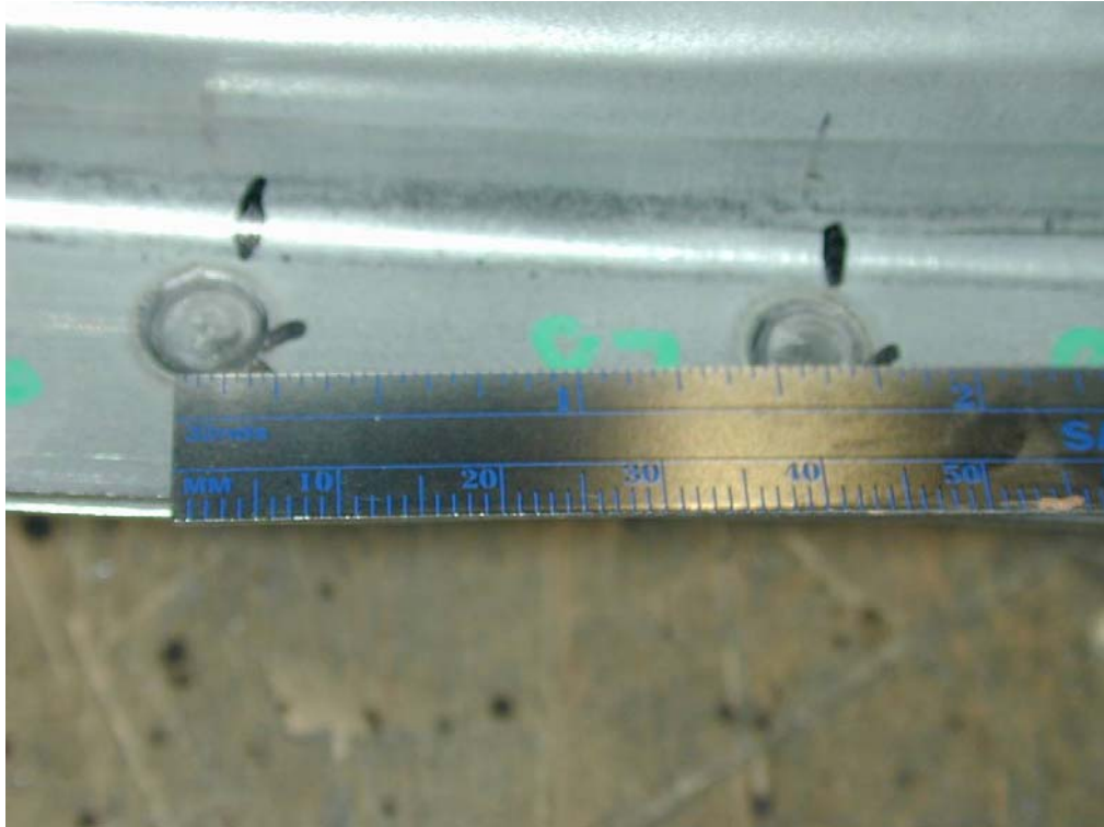
Photo 9. Pitch for spot welds from bumper attachment to end of tailor-welded blank.
