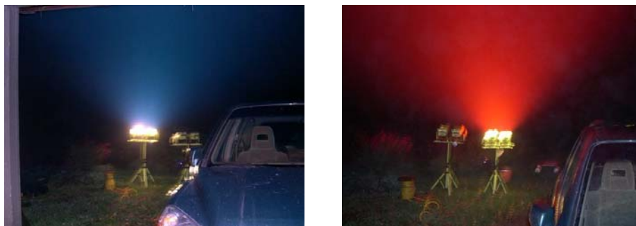
Fig. 1. 1500W halogen test lights with blue and red filters.
