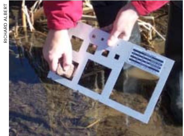
Measuring a stream particle with the AL-SCI Field Sieve/Gravelometer designed by Richard Albert.
