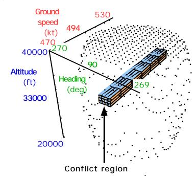
Fig 4. space and conflict region for the scenario of Maneuver Figure 3. The maneuver space is where the ownship could go, physically, given four minutes. The conflict region is where it cannot go, if its pilot wants to avoid a conflict with the intruder aircraft.
