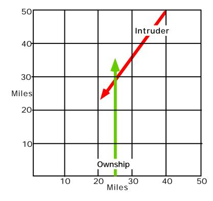
Fig 3. Map view of a prototype conflict. Both aircraft start at a range of 50 miles and proceed at 494 knots ground speed at 33000 ft. (.85 mach), flying level, resulting in an X-crossing and violation of their protected zones.
