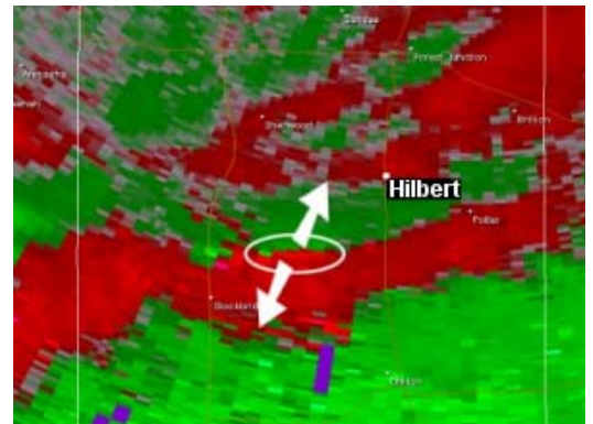
Doppler velocity image from the NWS Green Bay radar, taken at 11:56 pm on April 13. The arrows denote wind ("radial velocity") as seen by the radar. Area circled is strong divergence, a signature of a potentially damaging downburst.
