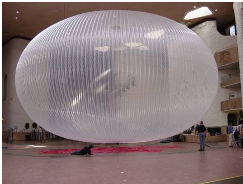
Figure 1. 14.3 m diameter, 200 gore model test balloon #10
