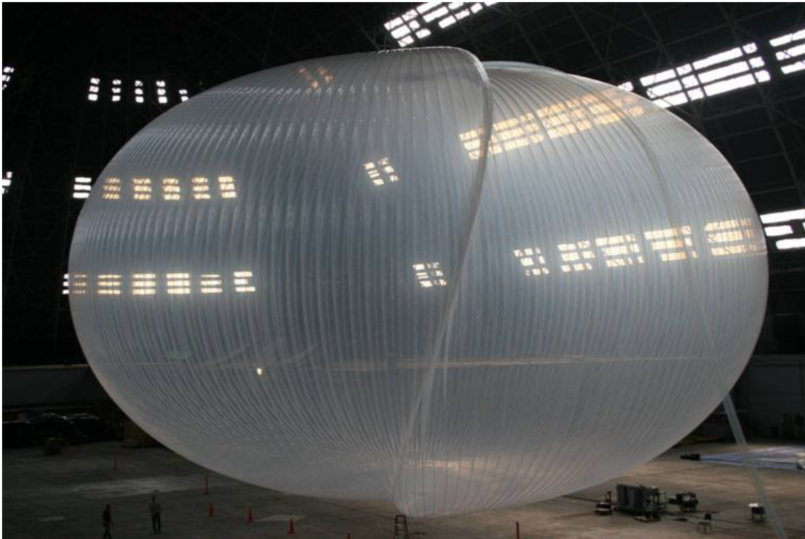
Figure 9. ~27m diameter balloon test replicating the “S” cleft seen in flight 555NT
