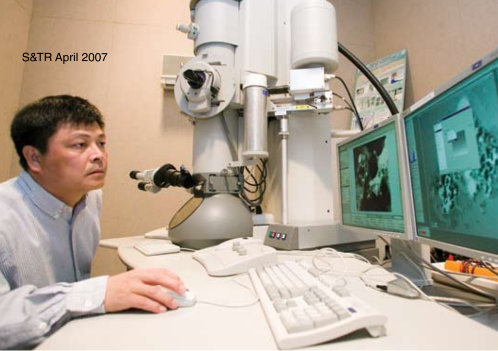
Zurong Dai uses a transmission electron microscope to take close-up images of cometary dust particles extracted from the aerogel cells.
