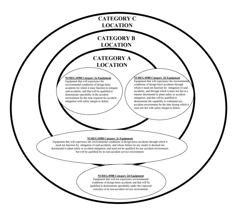
Figure 1. Pictorial mapping of the equipment categories identified in Appendix E of NUREG-0588 into the proposed location categories
