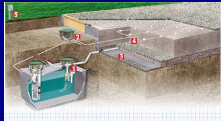
Recirculating Sand Filter
