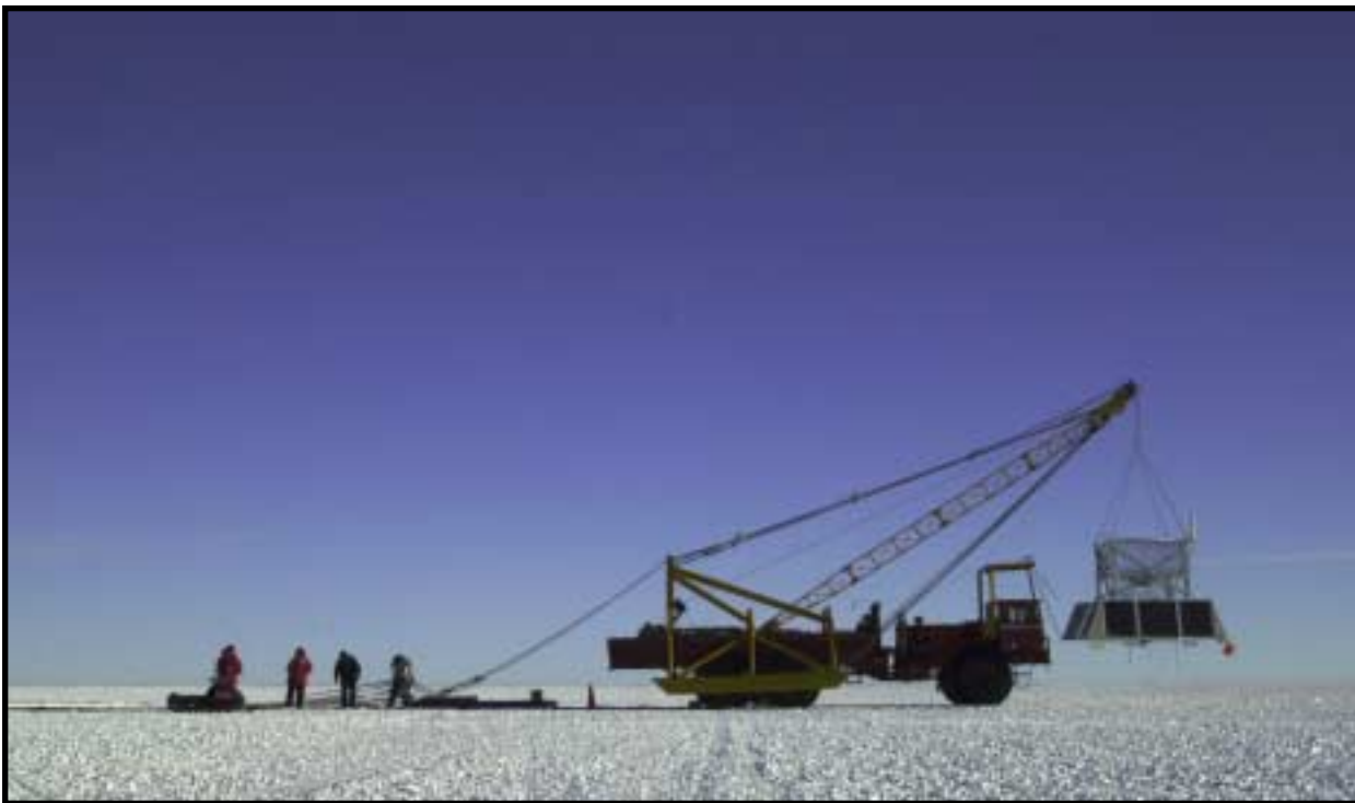
Workers lay the Long Duration Balloon into position with the science load on the front. The vehicle is used to pull the balloon once it is released to prevent it from falling to the ground.
