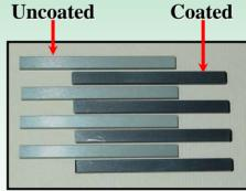
Pack cementation of AS800  $Si_3N_4$ bars in an Al -  $NH_4Cl - Al_2O_3$  pack at 1000°C for 5 hr. in Argon
