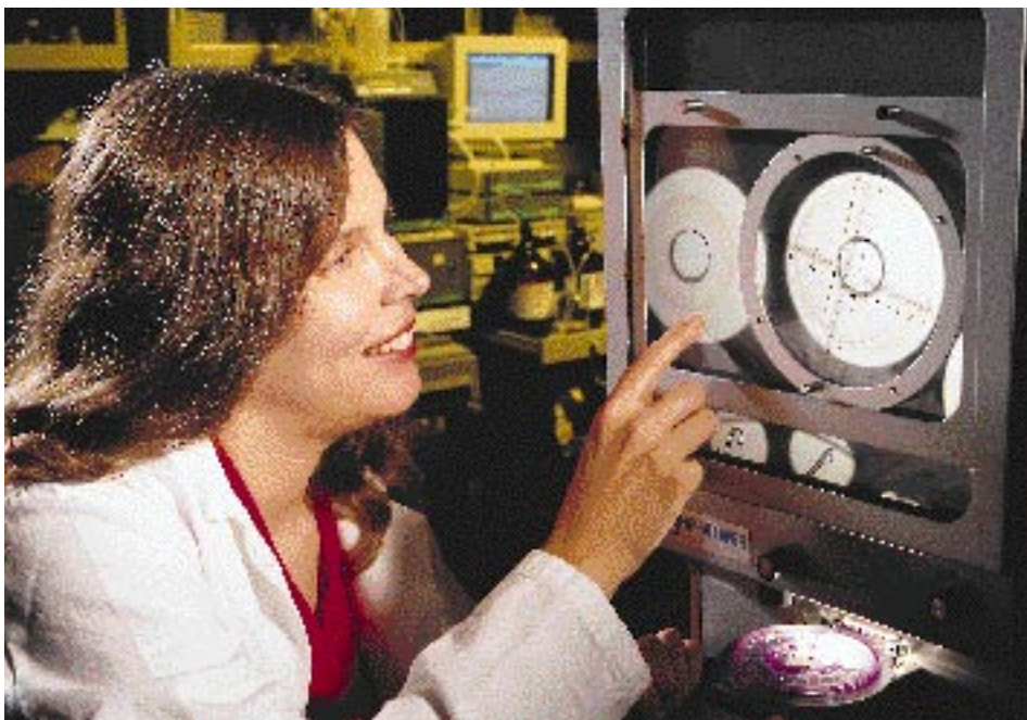
Rings shown on the plastic plate examined by ARS chemist Betty Burri reveal the amount of a vitamin-A-related protein in blood samples from volunteers. (K5755-3)
