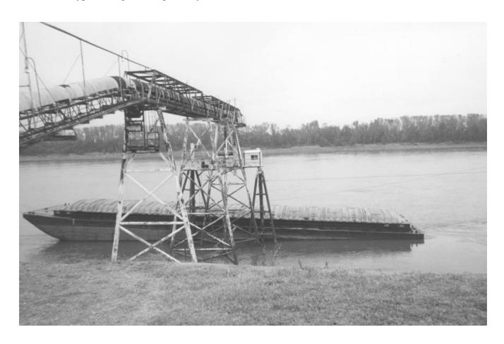
Photo 2. Continuous barge unloader.
