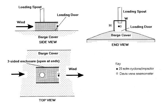
Figure 3. Sampling Deployment for Barge Loading Tests
