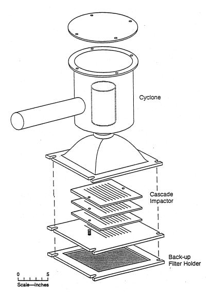
Figure 2. Cyclone Preseparator/3-Stage Cascade Impactor (20 acfm)
