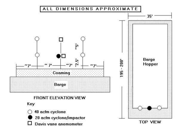
Figure 5. Sampling Deployment for Barge Unloading Tests
