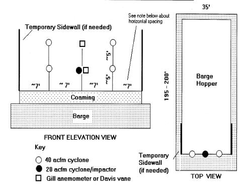
NOTE: Dimensions shown are for case in which sidewalls are used. If no sidealls are used, the "fenders" of the unloading station bound the horizontal extent and the spacing between samplers will be changed to again divide the sampling plane into quarters.
