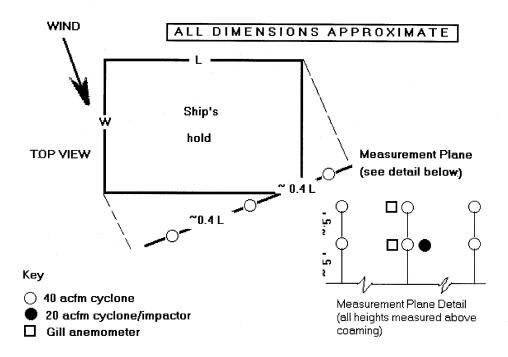
Figure 5. Sampling Equipment Deployment for Ship Loading Tests
