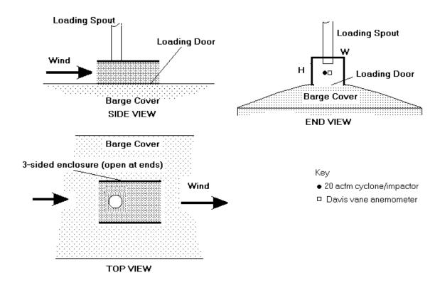
Figure 6. Sampling Equipment Deployment for Barge Loading Tests
