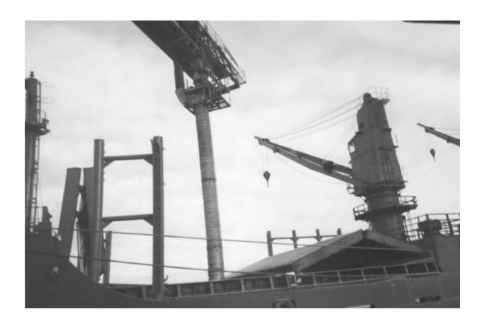
Photo 5. Sloped vessel (ship) loading spout.
