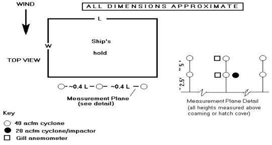
Figure 4. Equipment Deployment for Vessel (Ship) Loading Tests
