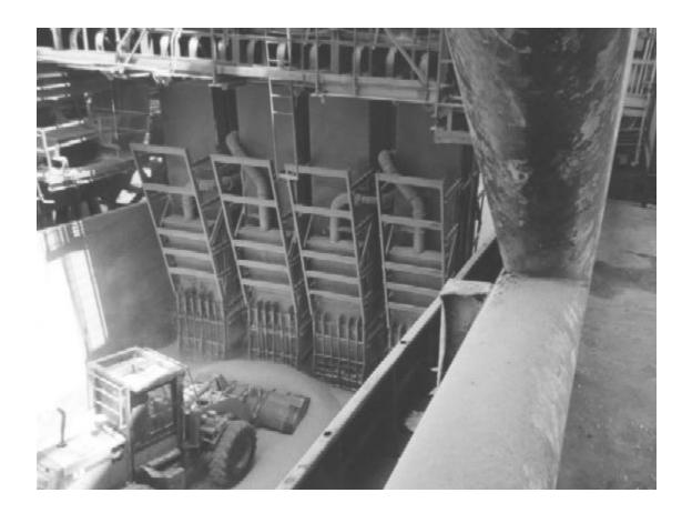
Photo 4. Straight vessel (ship) loading spout.
