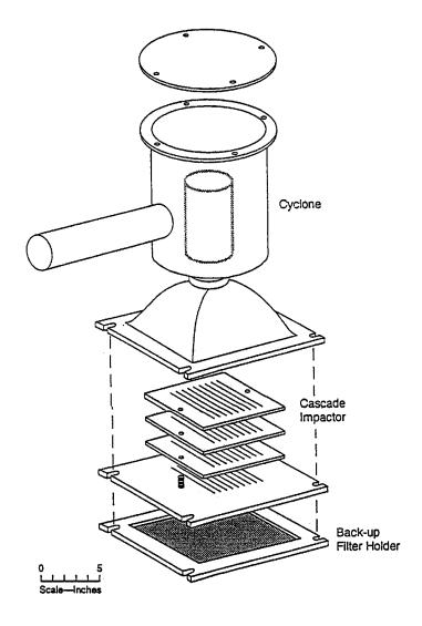
Figure 2. Cyclone Preseparator/Cascade Impactor (20 acfm)
