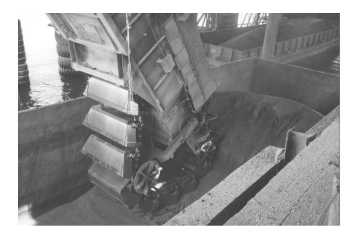
Photo 3. Marine leg barge unloader.
