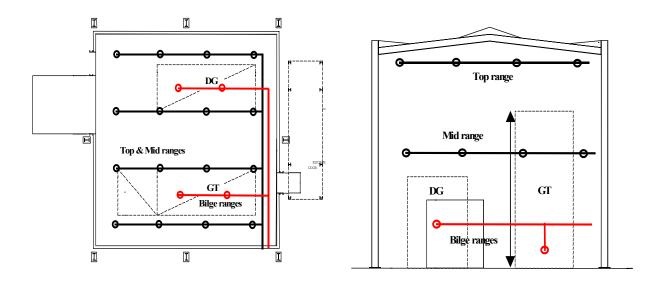
Figure 3 – Plan view of FWS pipe array in WSA's large scale test enclosure
