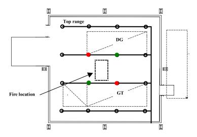
Figure 5 – Blocked nozzle locations
