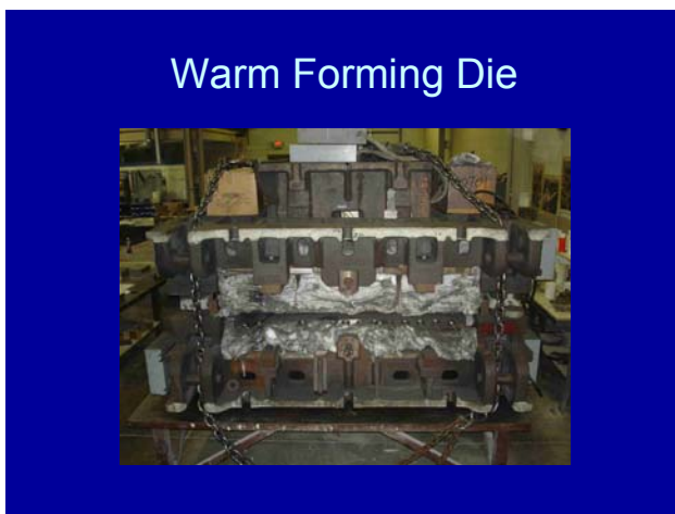
Figure 2. Picture of the warm-forming die constructed for the feasibility demonstration performed in Phase I.
