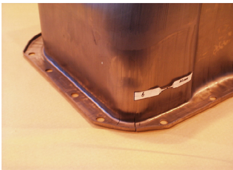
View of an oil pan showing cracking of a flange created during secondary forming operations
