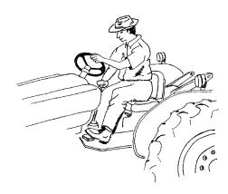
Without a ROPS and seat belt the operator is unprotected during an overturn.
