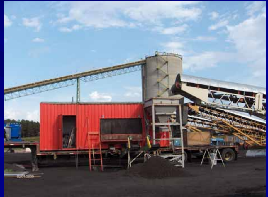
Mobile 5 tph FGX Unit and Test Setup
