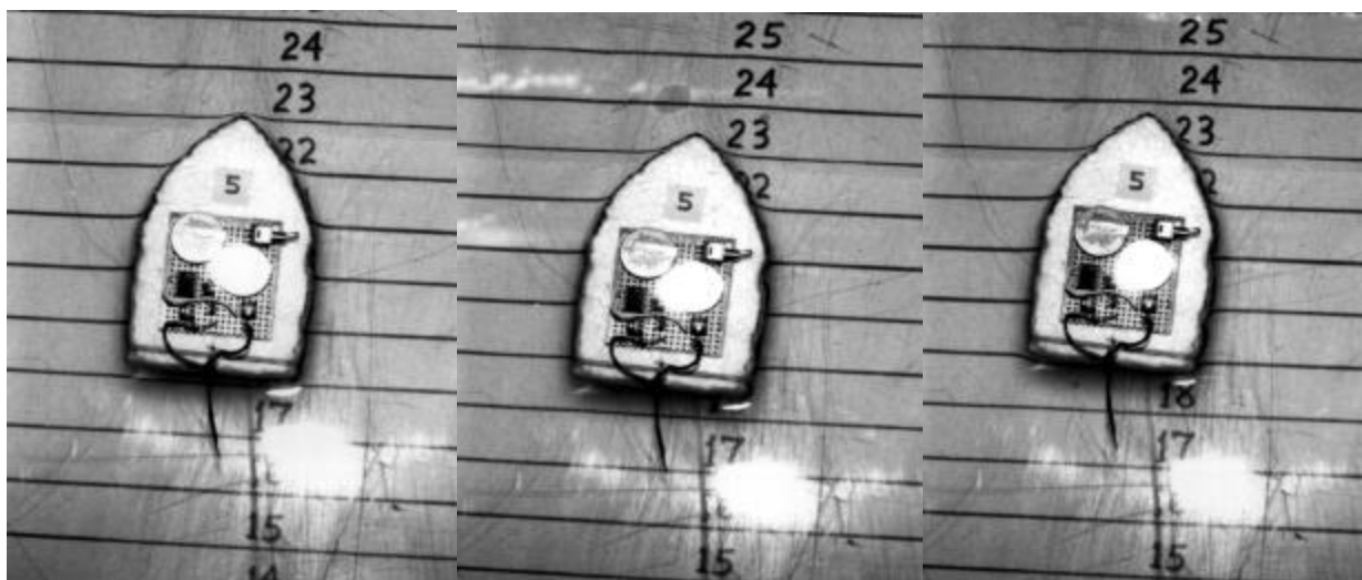
Figure 13. Robotic swimmer with muscle undulation frequency of 5 Hz (frame time interval, 1/3 second).
