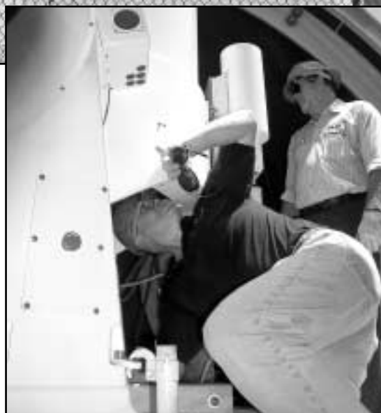
(Top inset) A worker looks at a five-meter (focal length) telescope being removed for repair. As part of the Distant Object Attitude Measurement System, the tracking telescope provides optical support for launches from Kennedy Space Center and Cape Canaveral. KSC-03PD-2673
