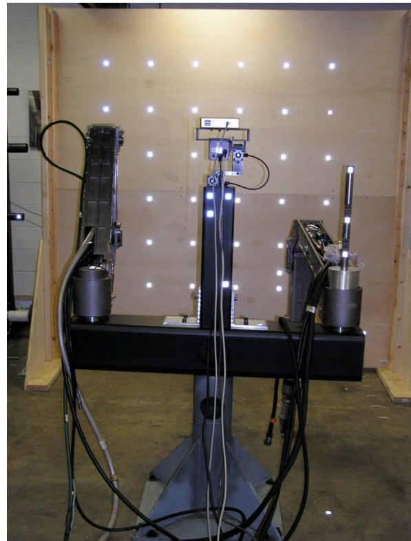
Fig. 4. Dual arm manipulator with calibration fixturing on the right arm, sensor head, and calibration array.
