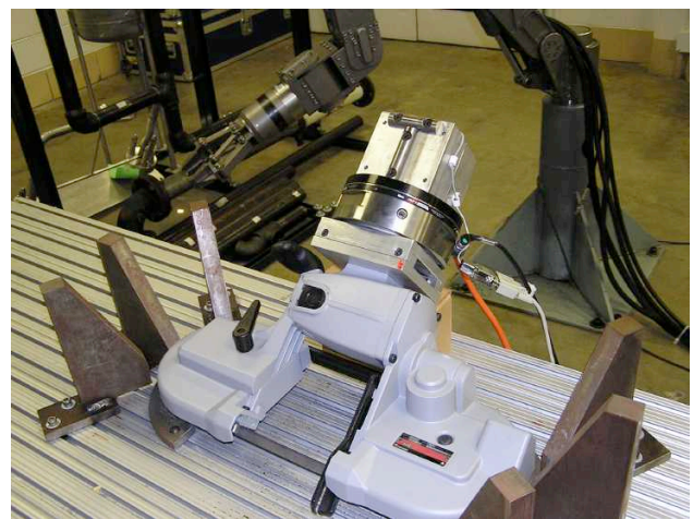
Fig. 6. Handheld band saw modified for parallel gripper use.
