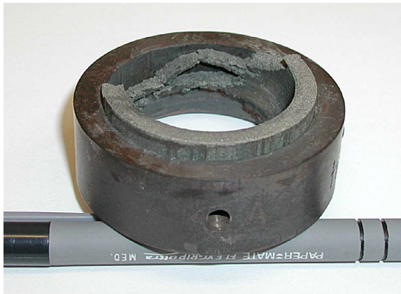
Figure 6.—Failed PM300 bushing under initial test conditions.
