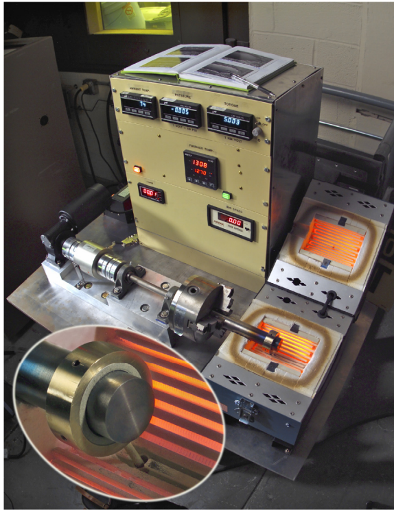
Figure 5.—High temperature PM300 bushing test rig.
