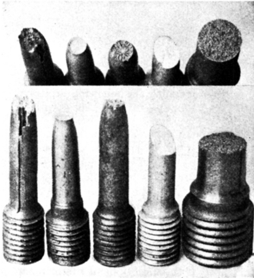
FIG. 16.10. Typical tensile fractures. (a) Wrought iron (ragged fracture showing slag). (b) Heat-treated alloy steel (perfect cup and cone). (c) Heat-treated alloy steel (rosette fracture). (d) Duralumin, heat-treated (shear fracture). (e) Gray cast iron (granular fracture). (Cowdrey and Adams, 1935. Courtesy of Wiley.)
