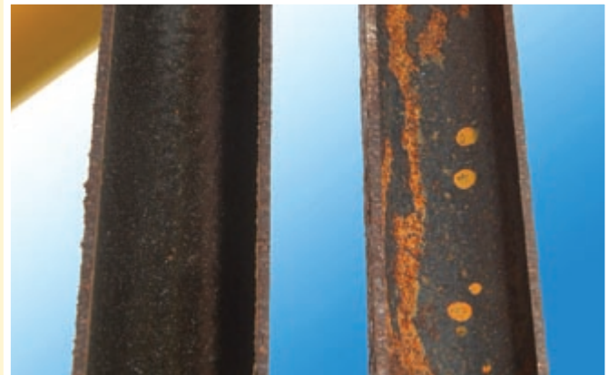
PPS coating on the left and a failed coating on the right.
