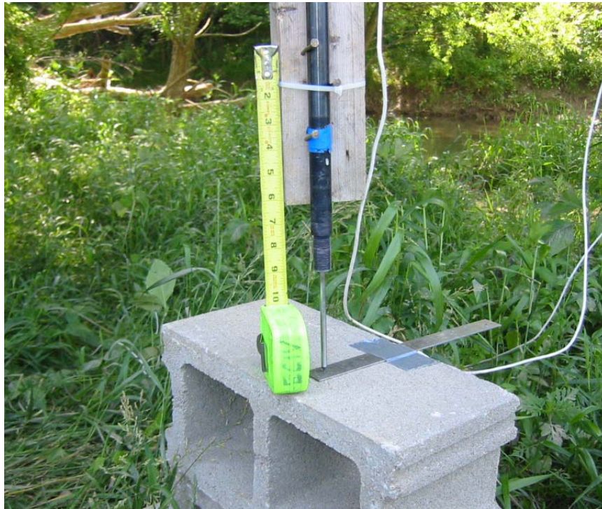
Figure 13. Displacement transducers to measure vertical deflection
