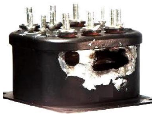
Figure 3-3. Damage from metal vapor arc
