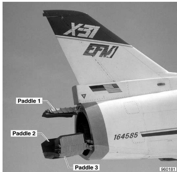
Figure 3. The X-31A thrust vector paddle arrangement.
