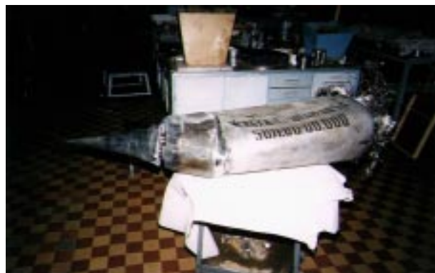
Figure 7. Recovered scramjet engine after flight.
