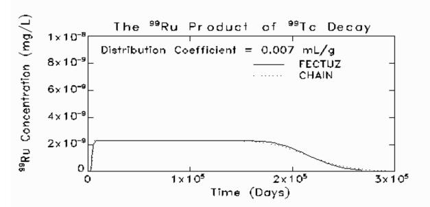
Figure 3.3. Base case simulations of the daughter product -- <sup>99</sup>Ru of <sup>99</sup>TC breakthrough (through the unsaturated zone) with a distribution coefficient of 0.007 mL/g using FECTUZ, and CHAIN models.
