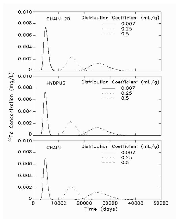
Figure 3.1. Base case simulations of <sup>99</sup>TC breakthrough (through the unsaturated zone) with three distribution coefficients using the CHAIN, <u>HYDRUS</u>, and CHAIN 2D models.
