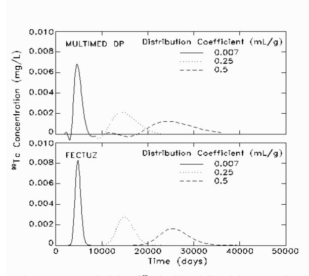
Figure 3.2. Base case simulations of <sup>99</sup>TC breakthrough (through the unsaturated zone) with three different distribution coefficients using the FECTUZ, and MULTIMED\_DP models.
