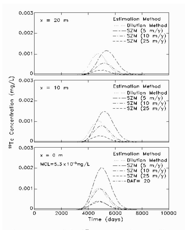
Figure 3.4. Base case predication of <sup>99</sup>TC concentration at the receptor well by employing dilution factor method and using saturated zone model (SZM) -- FECTUZ. The numbers in the parenthes2s are ground water velocity. The solid lines are used to represent the MCL ( $5.3 \times 10^{-5}$  ml/L) level.
