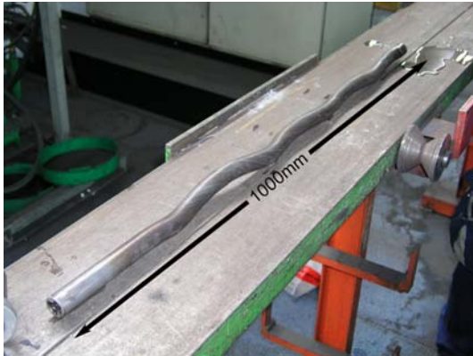
Figure 15 PM2000 tube twisted in commercial trials. Spiral buckling has occurred.
