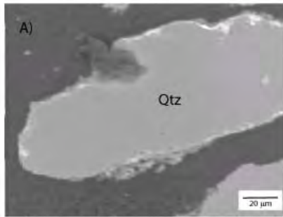
Back-Scattered Electron Image (BSEI) of a quartz grain in sample from well MAU-04. The grayscale gradients at the grain rim delineate the presence of a different phase.
