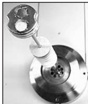
Cell mounting for typical heat-flux-type DSC system used for high-temperature applications.
