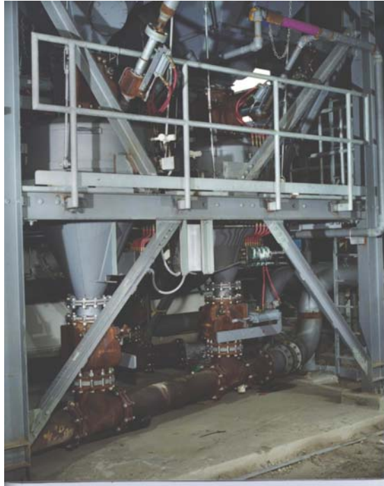
NUVAFEEDER Airlock vessels under Bed Ash transfer hopper
