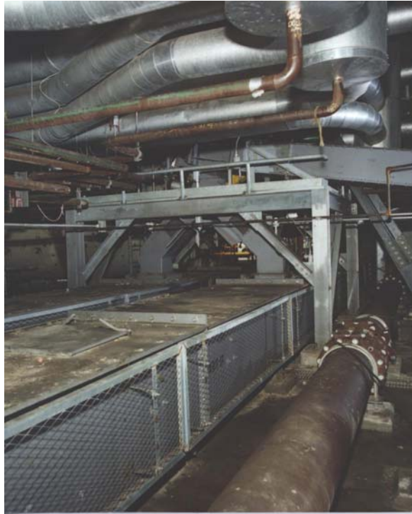
Bifurcated outlet of Stripper/Cooler drag chain feeding Gathering drag chain conveyors
