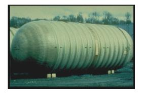
This is a picture of a fiberglass-reinforced **tank**. Notice the ribbing and rounded edges.
