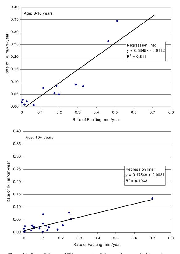
Figure 21. Rate of change of IRI versus rate of change of average faulting values.
