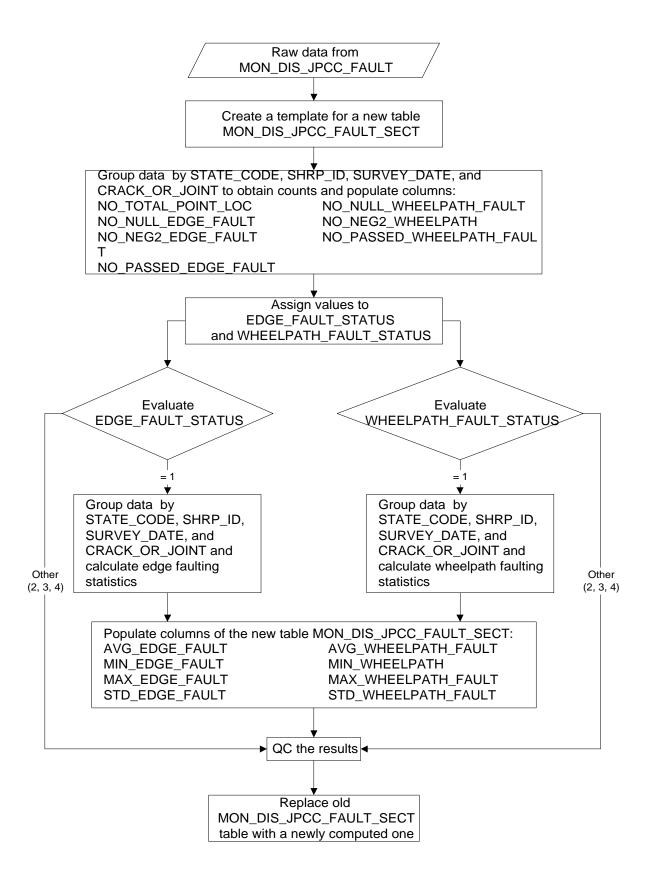
Figure 9. Flowchart for computation of faulting statistics.
