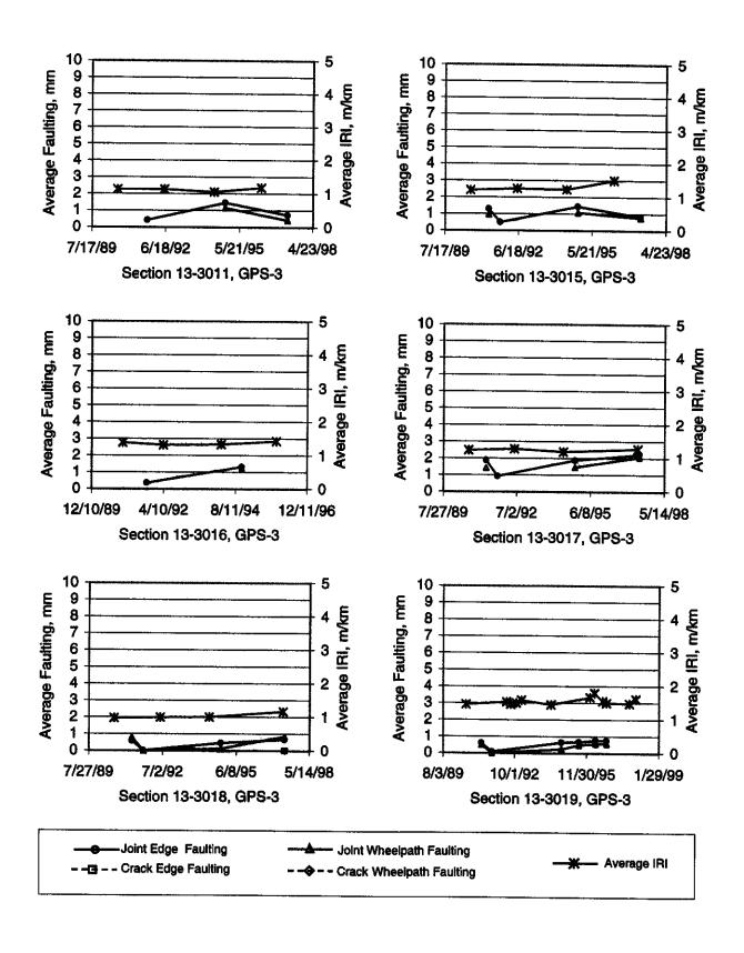
Figure 32. Time series plots for GPS-3 sections 133011, 133015, 133016, 133017, 133018, and 133019.
