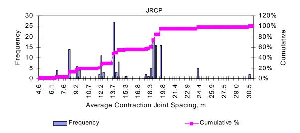
Figure 25. Joint spacing frequency distribution for different types of JCP.
