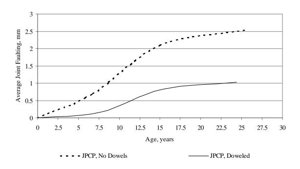
Figure 23. General trend of faulting development with time for doweled and non-doweled JPCP sections.
