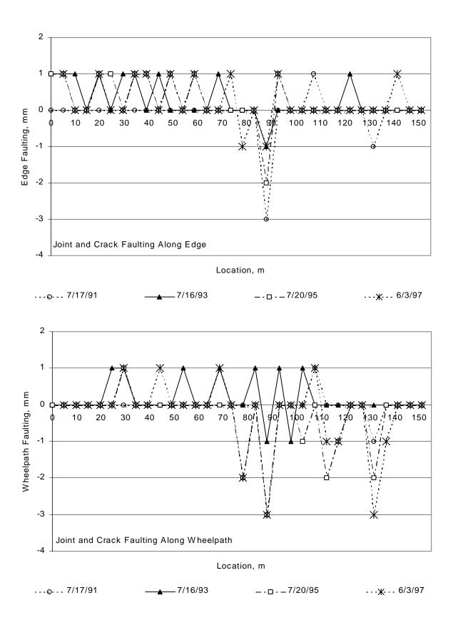
Figure 5. Example of consistent negative faulting (GPS-3 section 893016).
