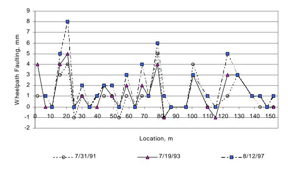
Figure 2. Example of faulting profile for GPS-4 section 314019.
