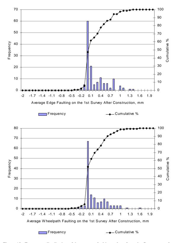
Figure 12. Frequency distribution of the average faulting values from the first survey after construction for SPS-2 sites.
