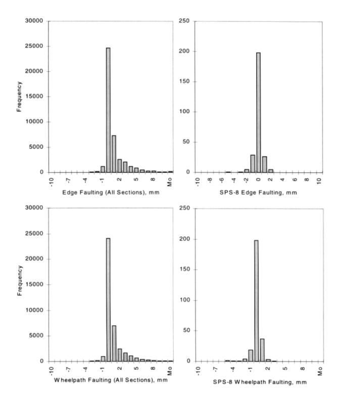
Figure 6. Comparison of faulting frequency distribution for sections subjected to traffic loading and sections without traffic (SPS-8 experiment).
