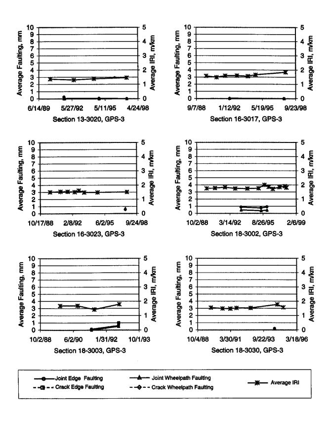
Figure 33. Time series plots for GPS-3 sections 133020, 163017, 163023, 183002, 183003, and 183030.
