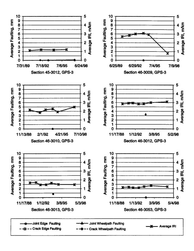
Figure 41. Time series plots for GPS-3 sections 453012, 463009, 463010, 463012, 463013, and 463053.
