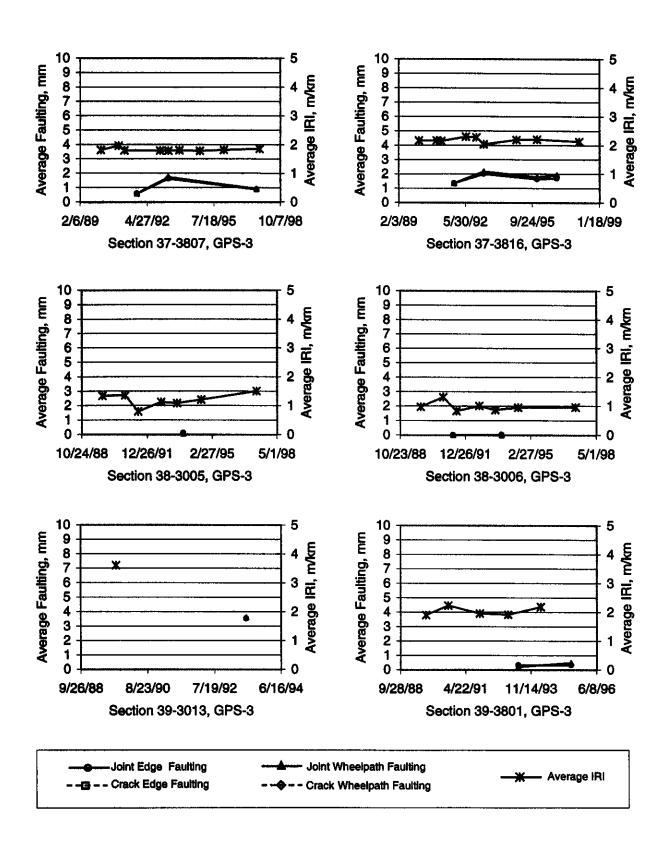
Figure 39. Time series plots for GPS-3 sections 373807, 373816, 383005, 383006, 393013, and 393801.
