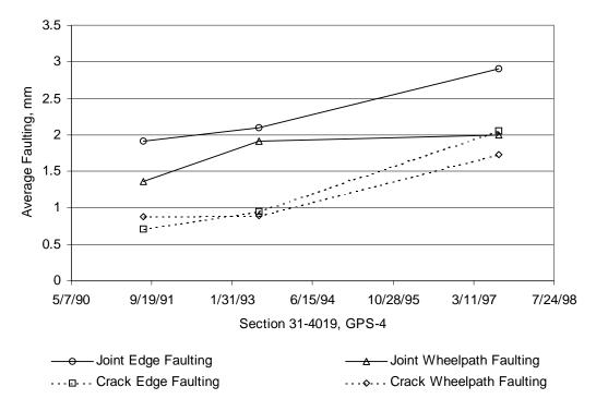
Figure 13. Example of a reasonable average faulting trend with time.
