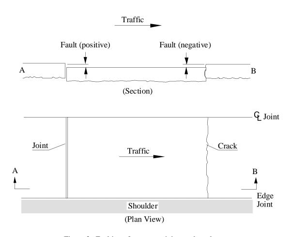
Figure 3. Faulting of transverse joints and cracks.
