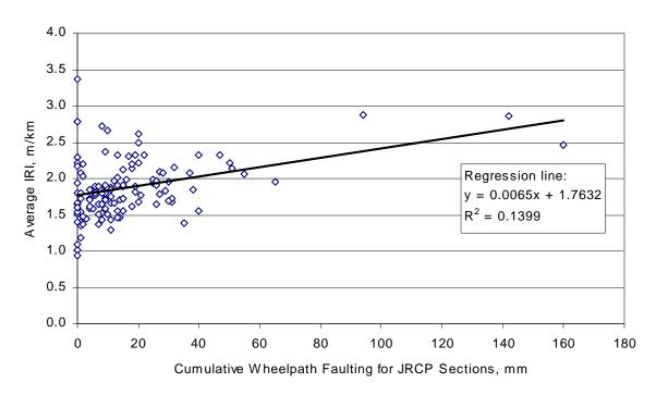
Figure 20. Cumulative faulting versus average IRI for JRCP sections (initial IRI not considered).
