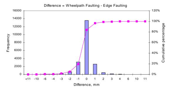
Figure 7. Frequency distribution of the difference between wheelpath and edge faulting data.
