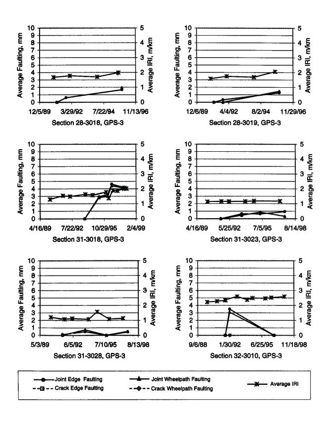
Figure 37. Time series plots for GPS-3 sections 283018, 283019, 313018, 313023, 313028, and 323010.
