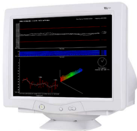
Figure 1. The Grid Monitor screensaver displays five graphs of real-time analyses of the AC power signal.
