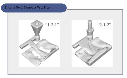
**G**ating trials to develop steel casting gating guidelines are ongoing. Further work is needed to understand the important factors in producing a good gating system. Graphics illustrate the effect of two different gating systems on metal flow into a small test plate.
