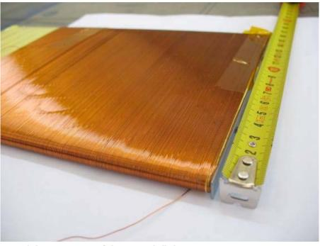
Prototype of the ex-vessel tangential coil located in area of large VV curvature.
