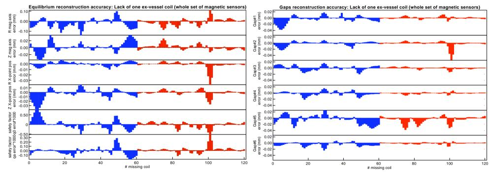
Simulation with all sensors (in-vessel coils, divertor, flux loops and ex-vessel coils). Error due to suppression of one ex-vessel coil assessed: **blue tangential** (1-60), **red radial** (61-120) Right-hand figure:  $R_{mag}$ ,  $Z_{mag}$ ,  $R_X$ ,  $Z_x$ , q; left-hand figure: gap 1-6. All in mm.
