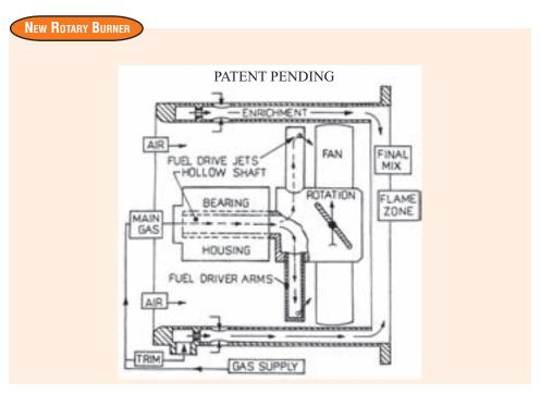
The new rotary burner provides fuel and electricity savings by using a gas expansion technique to mix air and fuel for combustion.
