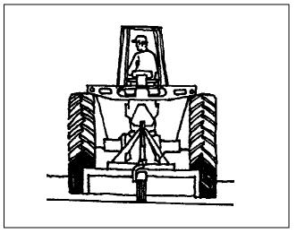
Figure 1. Keep wheels wide for tractor stability.
