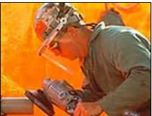
Face shield windows are made with different transparent materials and in varying degrees or levels
