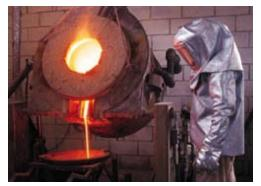
shield window should be matched to the task. Window and headgear devices come in various styles in order to enable the worker to select the appropriate equipment.
