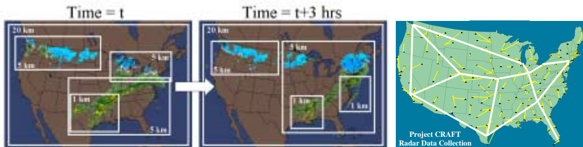
Figure 1. Dynamic nature of mesoscale prediction: the nested domains in left two panels change with time as the weather evolves. Abilene/I2-based system that feeds NEXRAD Doppler radar and other data to the forecast grids must adapt to dynamically evolving bandwidth requirements to ensure quality of service.
