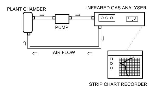
Fig. 3: Diagram of a closed CO<sub>2</sub> exchange system used to measure apparent photosynthesis and dark respiration.
