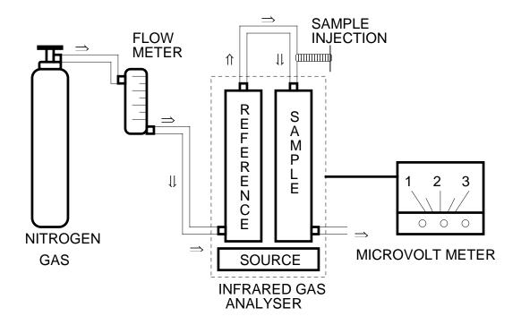
Fig. 2: Diagram of the CO<sub>2</sub> measurement system in the laboratory.
