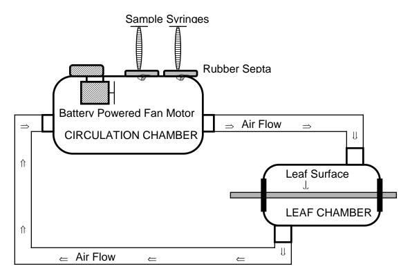
Fig. 1: Diagram of the closed CO<sub>2</sub> measurement system using the syringe technique to obtain CO<sub>2</sub> samples in the field.
