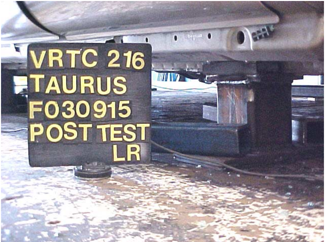
Figure A-42 Post-Test Left Rear Stand and Reinforcement View
