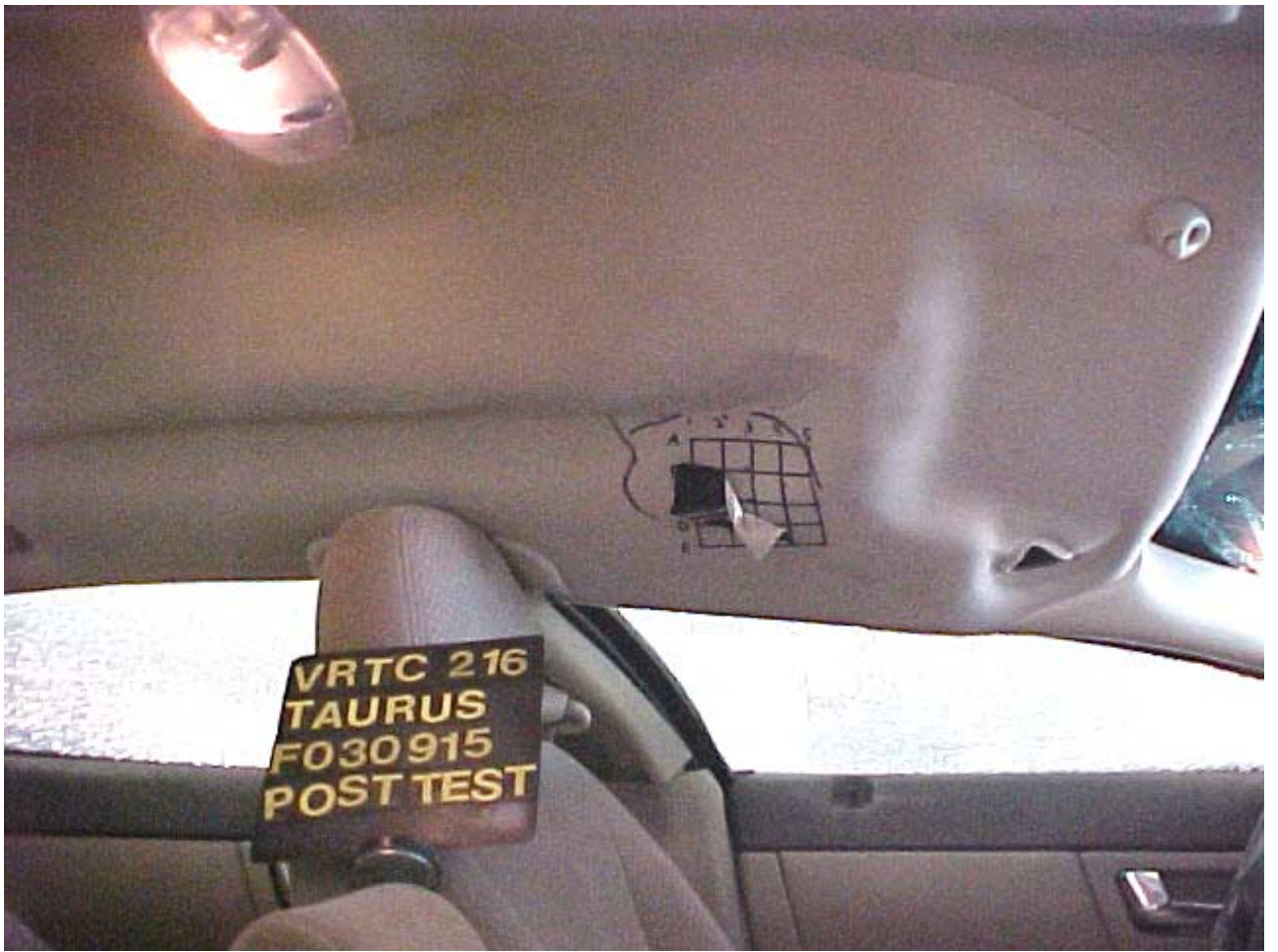
Figure A-45 Post-Test Interior Roof – View 1
