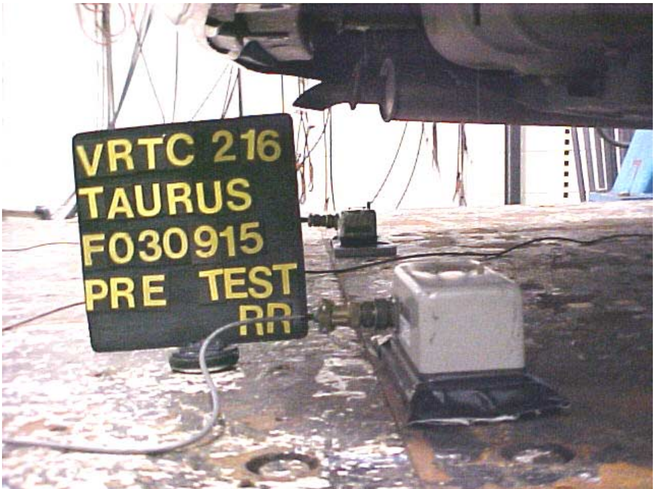
Figure A-20 Pre-Test Right Rear Displacement Potentiometer View
