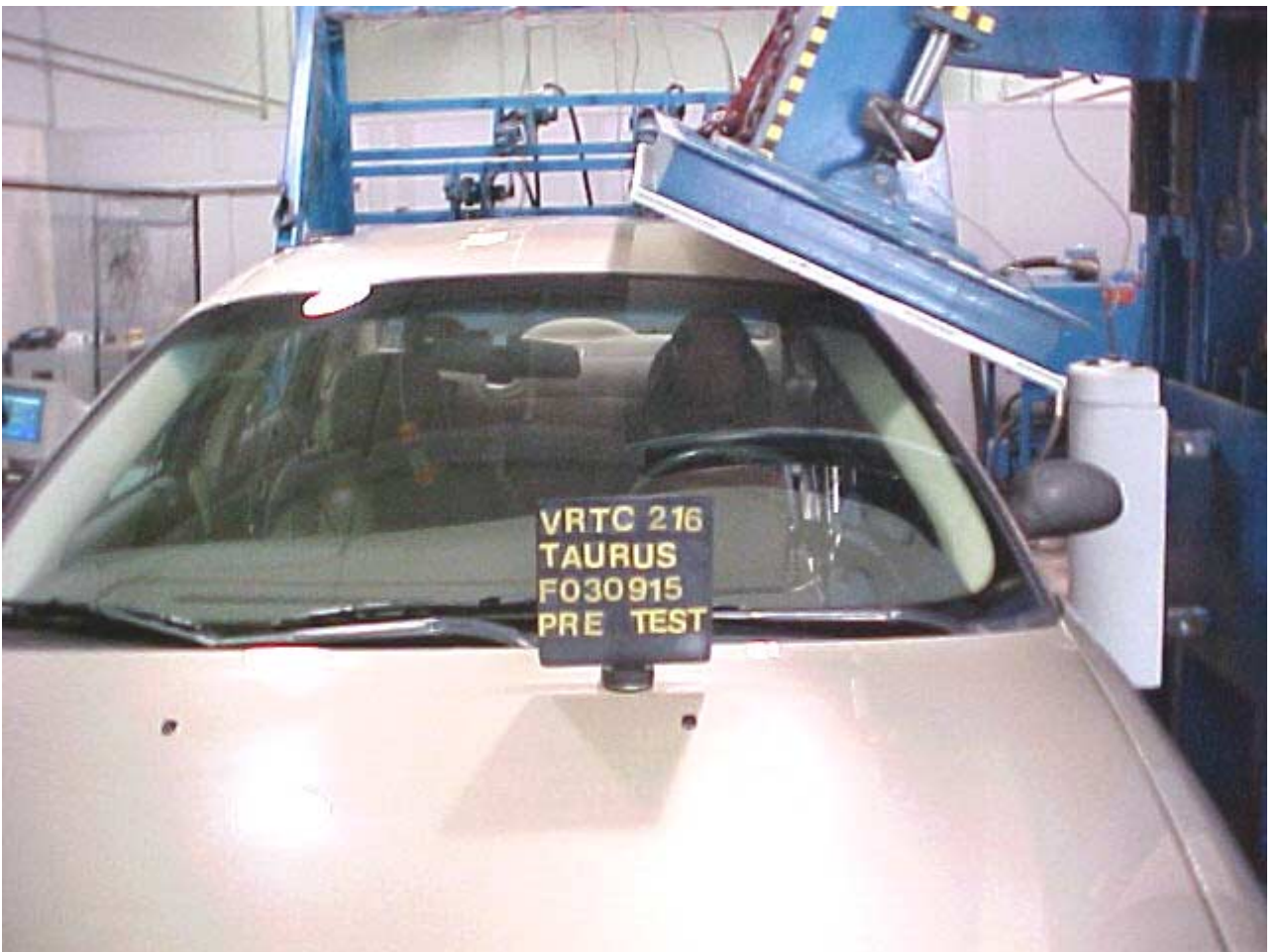
Figure A-12 Pre-Test Loading Device Initial Contact Point View
