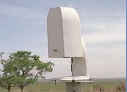
Measure cloud-base height at up to three levels. Maximum vertical range of 25,000 ft.
