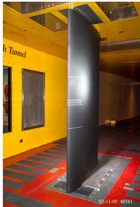
Figure 2.—91.4-cm-chord, 183-cm-span fiberglass NACA 0012 airfoil models installed in IRT test section.
