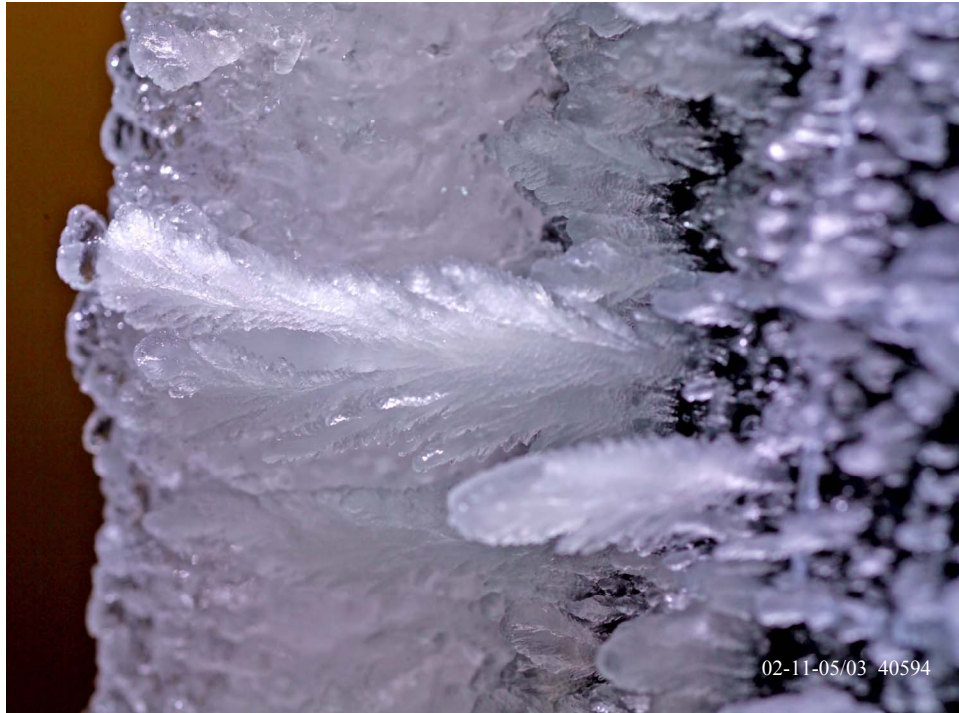
Figure 9.—Lower surface horn aft plane and feather region at the completion of the spray of figure 8. 02-11-05 Run 3. c , 91.4 cm; V , 100 kt; MVD , 30 \mu\text{m} ; \beta_0 , 69 percent; \beta_0 A_c , 1.80; n_0 , 0.50.
