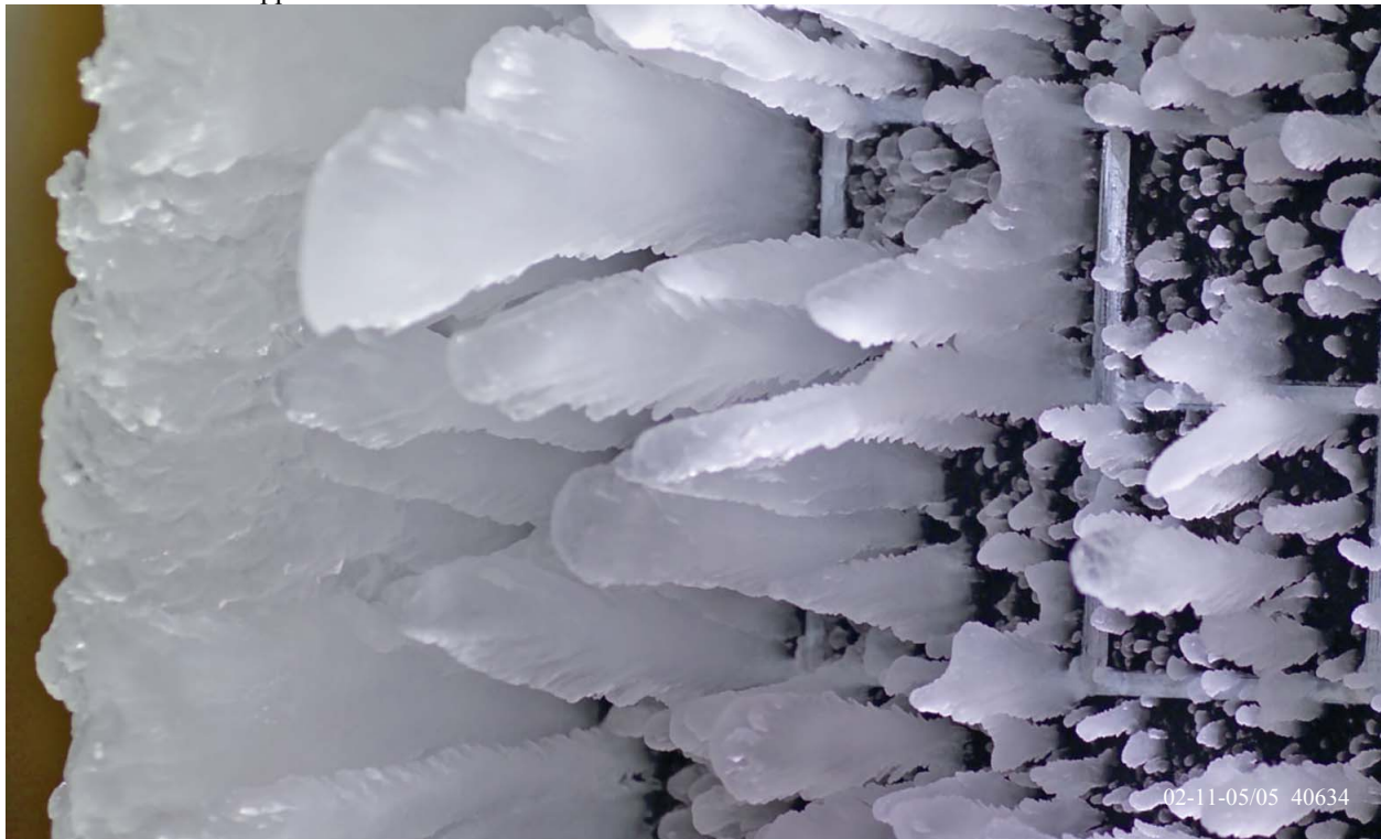
Figure 7.—Feather region and aft plane of horn on lower surface at the completion of the spray of figure 6. 02-11-05 Run 5. c , 91.4 cm; V , 100 kt; MVD , 140 \mu\text{m} ; \beta_0 , 94 percent; \beta_0 A_c , 1.80; n_0 , 0.50.
