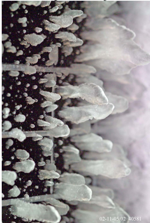
Figure 5.—Feather region and aft plane of horn on upper surface at the completion of the spray of figure 4. 02-11-05 run 2. c , 91.4 cm; V , 100 kt; MVD , 140 \mu\text{m} ; \beta_0 , 94 percent; \beta_0 A_c , 1.80; n_0 , 0.30.
