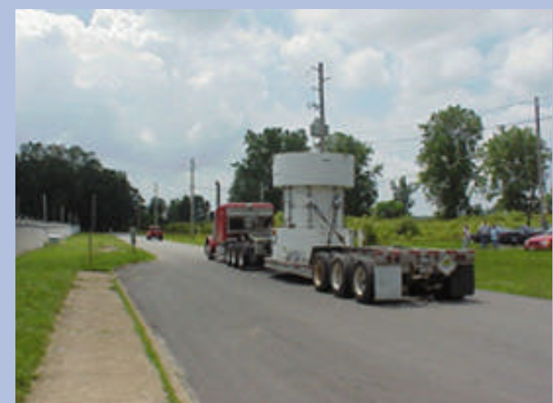
A steel liner containing segmented reactor internals is placed in a shipping cask (left). The cask sits on a flatbed truck as it leaves Plum Brook Station for the Barnwell licensed disposal facility in South Carolina.
