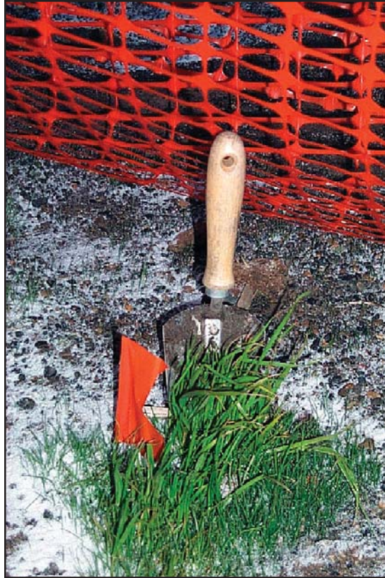
Fescue and ryegrass growing on petroleum-contaminated soil in test plots near the Naval Arctic Research Laboratory site at Barrow, Alaska.
