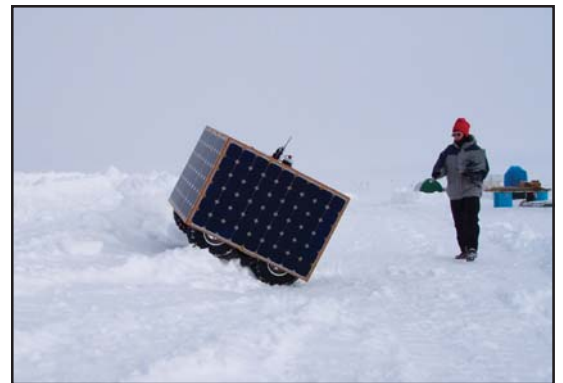
Cool Robot climbing a 0.3-m-high, steep-faced snow berm at Summit Camp, Greenland.
