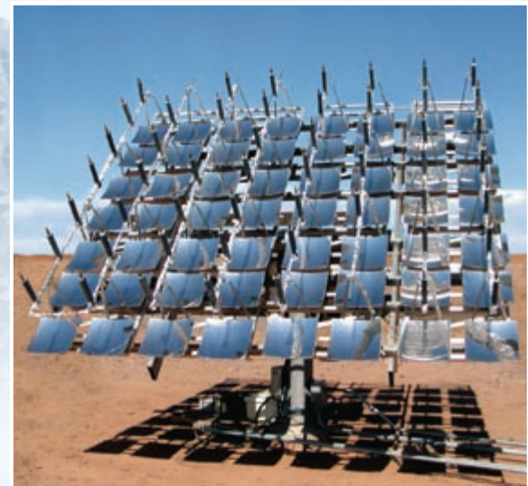
Concentrators such as this one focus sunlight onto high-efficiency multijunction PV cells.
